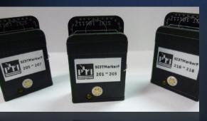
Wireless Self-Contained LED Markers - 6DOF unit with 3 LED targets
